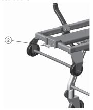
Z-Roller allows the housing of a cot for the resting on special profiles as shown in the following images.
