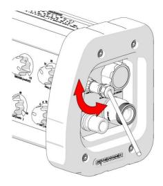
If you wish to wire the cable to the mains power of the ambulance, remove the plug, splice and connect according to the specifications in the table.
