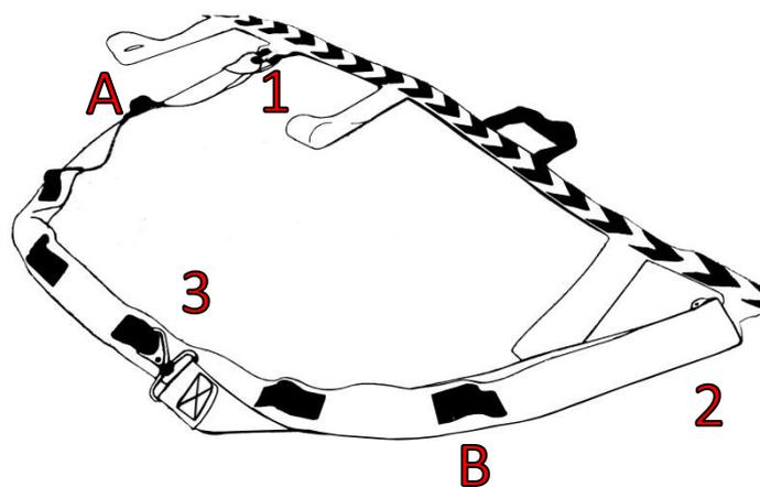
The shoulder strap can be adjusted in 6 positions by varying the loop on which the terminal carabiner is attached.
