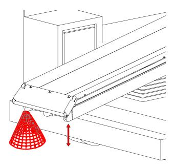
Innovative and patended system which automatically adjust the loading height of the stretcher support according to the conditions of the terrain and of the vehicle load. This accessory is factory installed upon request and is compatible with stretcher supports which can be extracted in tilted position.
