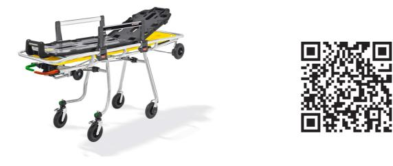
Carrera Pro is a self-loading stretcher for patient transport usable in rescue operations on streets and rescue vehicles. The legs fold away independently, activating the dedicated commands and they open automatically during the unloading procedure. The spinal board can be placed in a dedicated housing located under the patient board.
