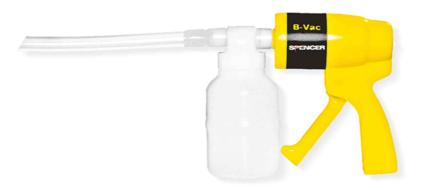
Manual aspirator for secretions with reduced obstruction capacity, its function is the removal of fluids from respiratory tracts or from the respiration support system and of infective material from wounds. The aspirator creates a depression which pulls fluids out through the disposable catheter tied to the disposable vessel. It does not need power source
